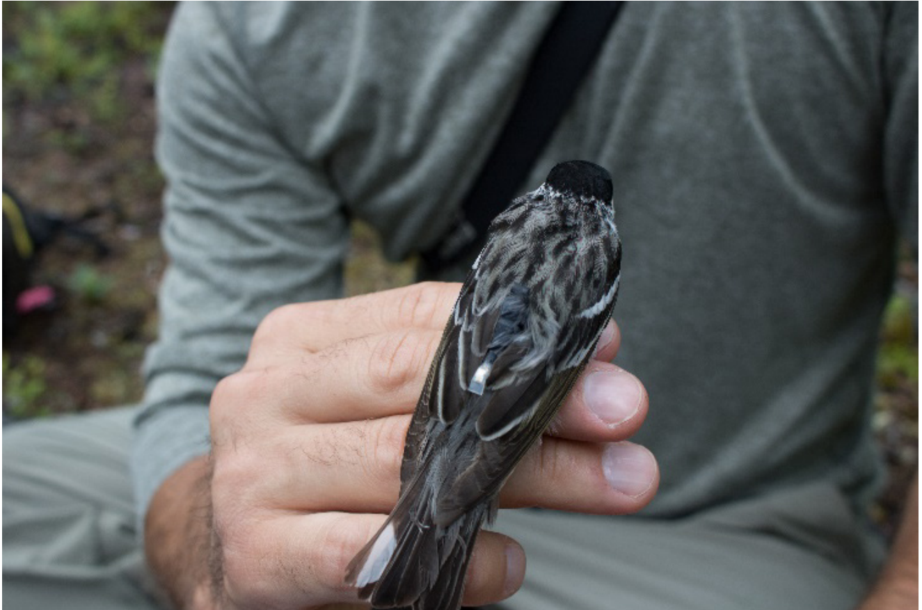
Photo 2. A male blackpoll outfitted with a light-level geolocator near Whitehorse, Yukon Territory, Canada. The light-sensing stalk is visible, rising gently from the bird's back. The device records and stores the time, date, and light exposure every few minutes for up to a year. From this information, researchers can estimate, within a few hundred kilometers, where the bird moved throughout its annual cycle for that year. Photo credit: Hilary A. Cooke.
